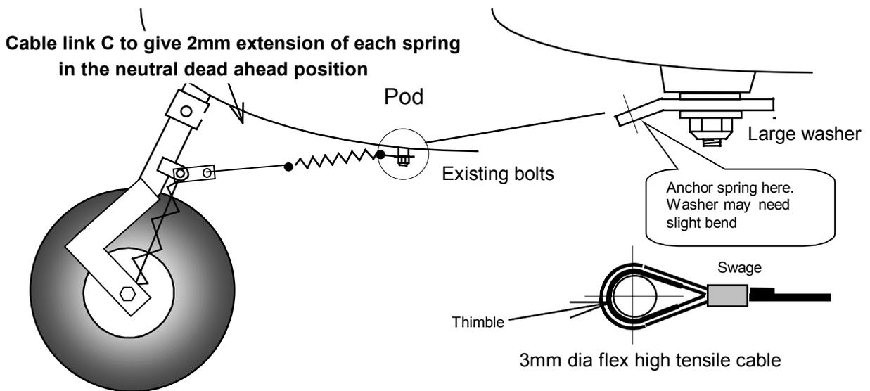
There are two 8mm bolts under the pod which locate and fix the rudder pedals. These may be used as anchor points for the links onto which the springs may be mounted. There are two large washers pre - drilled in the kit for this.
