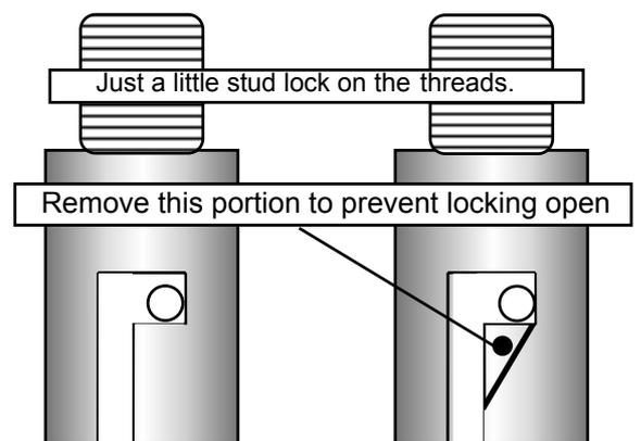
These threads are tapered, so when tightening, be careful to tighten just enough to seal using an AF spanner. Assemble the threads with a little stud lock. Tighten the whole assembly firmly. Over tightening may cause movement of the inserts moulded into the tank. Access will be needed below these cocks through the fabric to allow petrol and water
