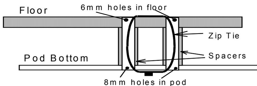
**Floor plan for drilling.** Go through floor and pod with a long 6mm dia.drill, deburr, insert spacers, locate zip tie and tighten. The tube spacers do not need to be accurately positioned, but get as near to the dimensions as you can, but not too near the edge so as to interfere with the operation of the sticks in the most forward position.
