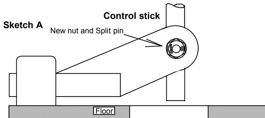
Drill and split pin both pilot and passenger control stick pivot bolts. Replace the nuts supplied with the 6 mm stainless steel nyloc nuts in the mod kit. This will give extra length of thread for drilling the split pin holes. Castlated nuts may be used if you wish. Split pins in mod kit.
