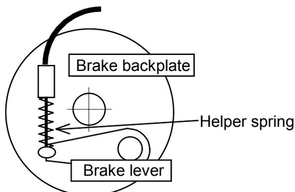
Make sure you disassemble the brakes, as I found they are packed dry. They will need a little Molydysulphide grease in the pivots and cam mechanism. **Make sure the brake pedals are free, it is possible to over tighten the elevator cable nut, crush the spacer, and stiffen the pedal movement.**
