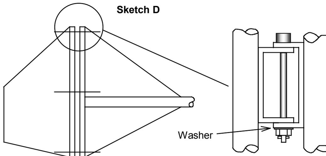
There are 7 of this hinges to be split pinned for the rudder and tail
