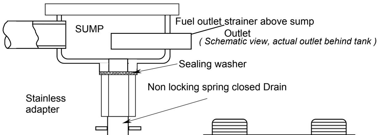
Two drain Cocks are provided in the kit, but they need modifying, as in the diagram in order to prevent them being locked open.
