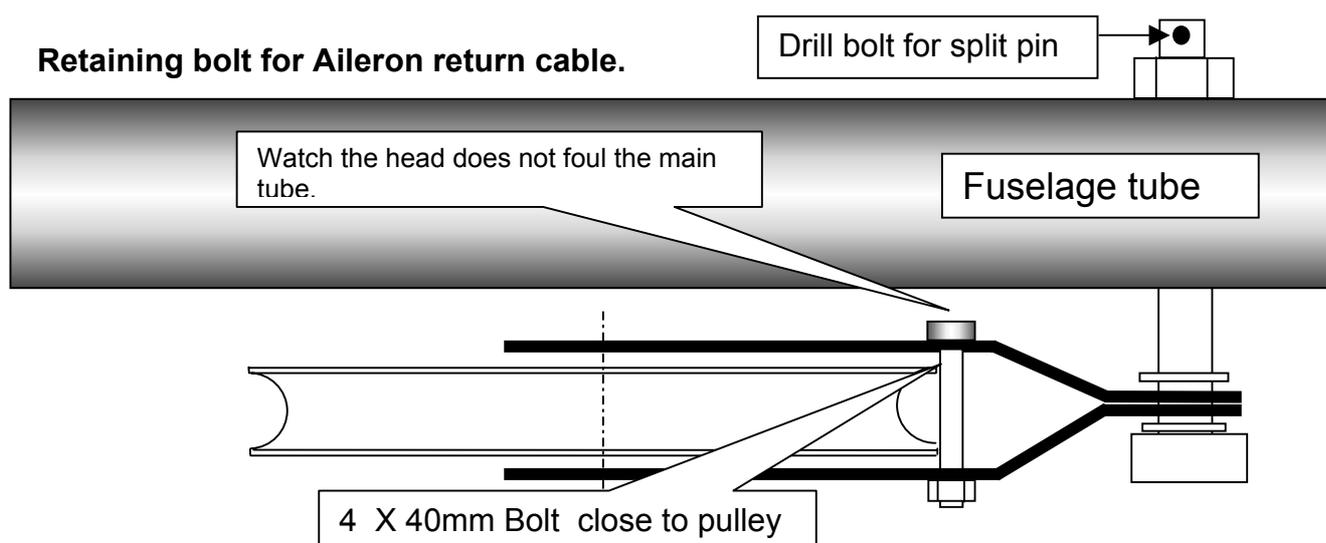
It may be possible on some aircraft for the cable of the Aileron return cable to jam down beside the pulley and the support bracket, particularly when assembling the final stages of the control systems.
