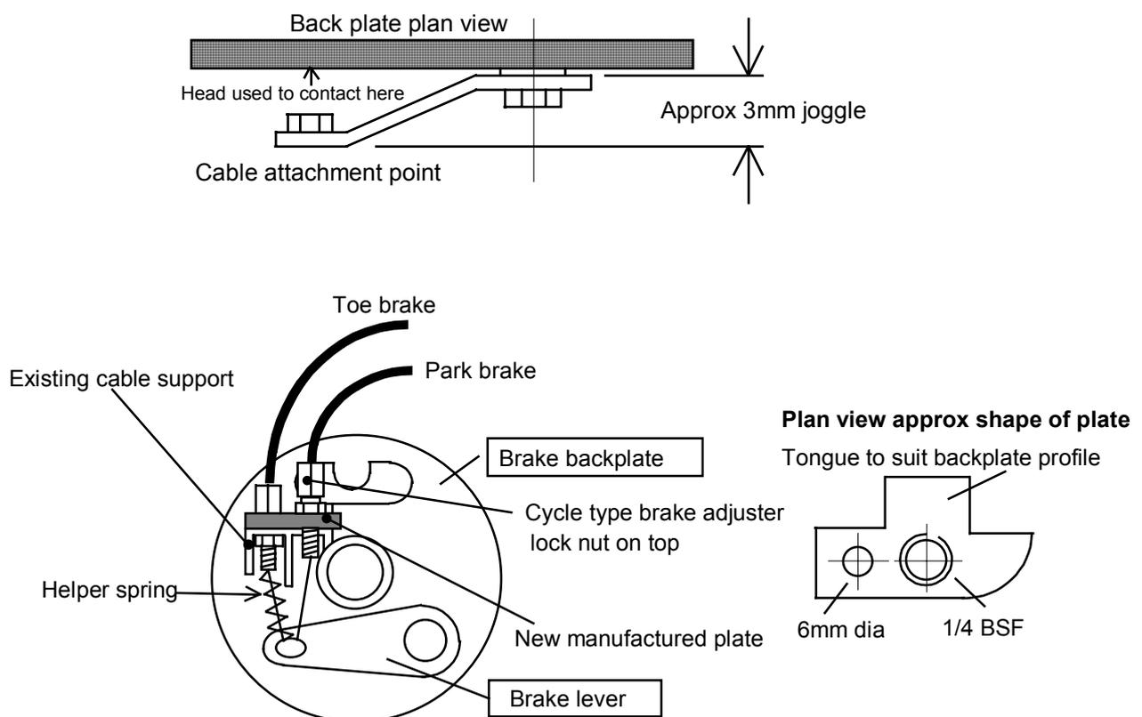
**Number 19** *Do this when all adjustments have been made to steering, rudder cables etc. .*
