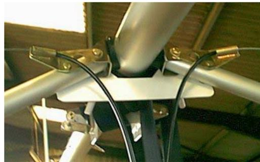
*Note's:- Fit a 6mm washer between Aileron cable brackets and tube 240.
