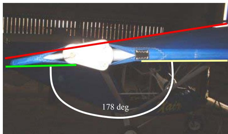
Set both aileron turnbuckles so that the stick is in the middle. Then adjust the aileron return cable turnbuckle so that the cables are taut, but not so tight as the stick is too stiff to move.
